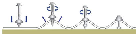
**Note:** For best performance use a variable speed drill. Before applying, ensure the cutting saw is seated firmly underneath the rubber washer.
